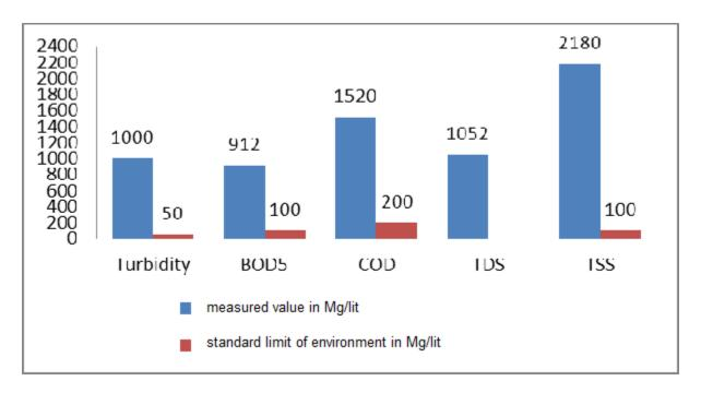
Fig. 2. Comparison of parameters of contaminants of exiting wastewater with the standards of Environmental Protection Organization of Iran for irrigation purposes.
