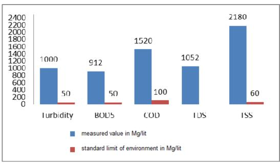
Fig. 3. Comparison of parameters of contaminants of exiting wastewater with the standards of Environmental Protection Organization of Iran for disposal in surface waters.
